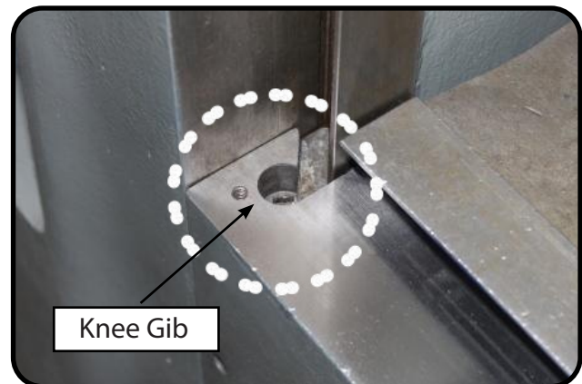
FIG. 31 KNEE GIB ADJUSTMENT
